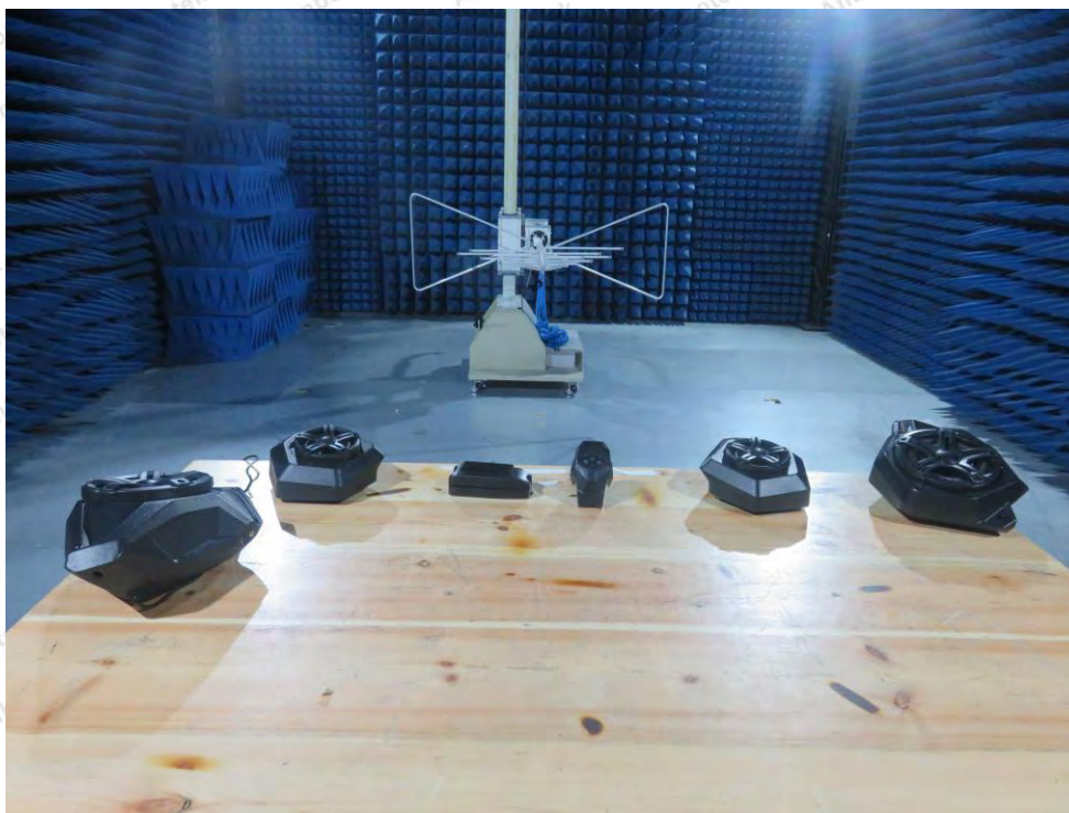
Photo of Radiation Emission Test
