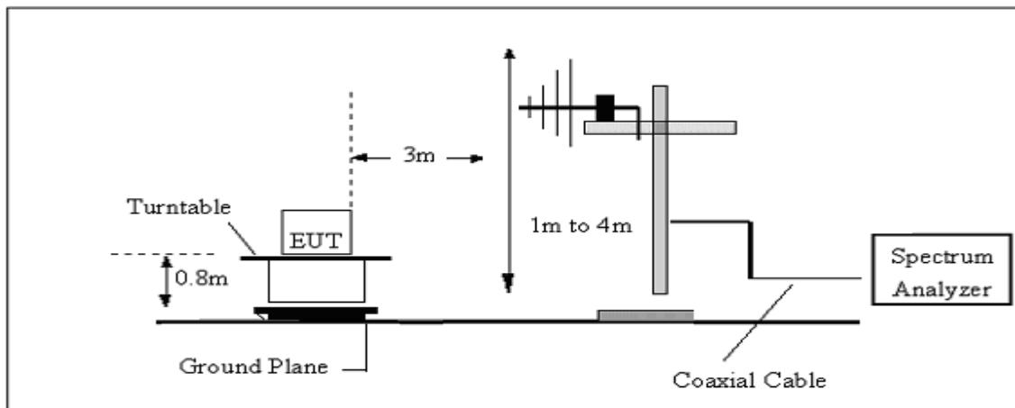
(B) Radiated Emission Test-Up Frequency Above 1GHz
