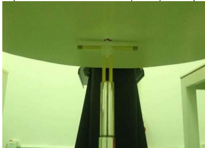
Photo of Dipole Setup
