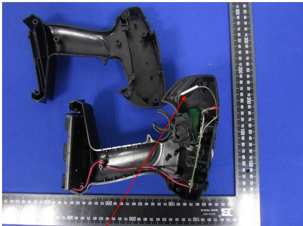
This is a Integral Antenna, antenna gain is 2.5dBi.
