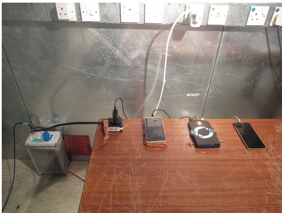
Set-up for AC Mains Conducted Emission (Charging + Discharging mode)
