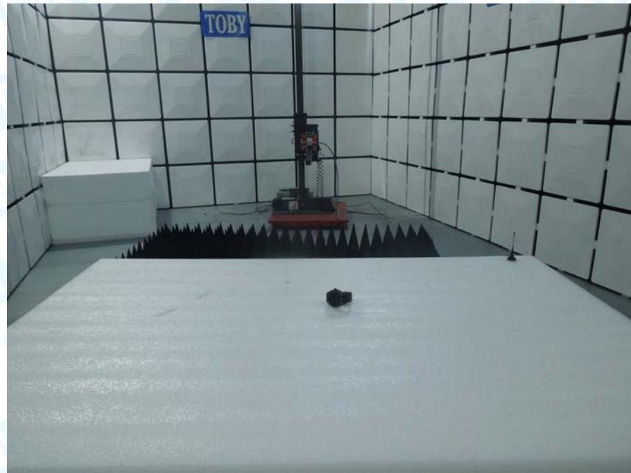
**Photo of Setup for Radiated Emission (Below 1 GHz)**
