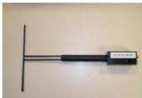
Figure 1 – Satimo COMOSAR Validation Dipole
