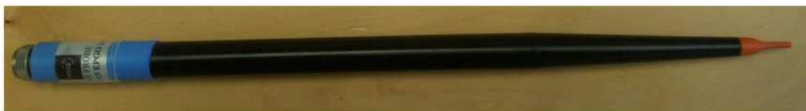
Figure 1 – MVG COMOSAR Dosimetric E field Dipole
