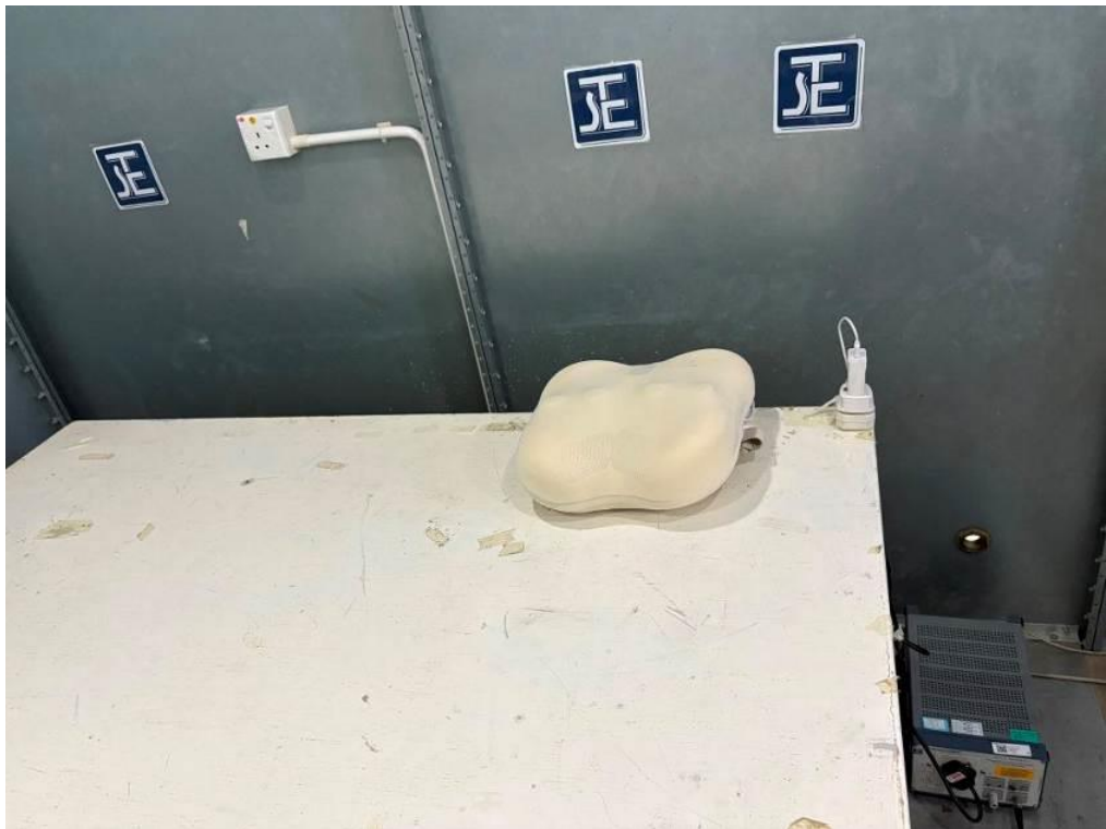
Measurement of Conducted Emission Test Set Up
