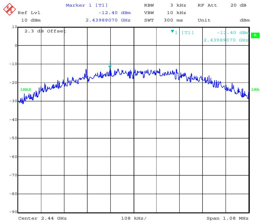
**Power Spectral Density, High Channel**
