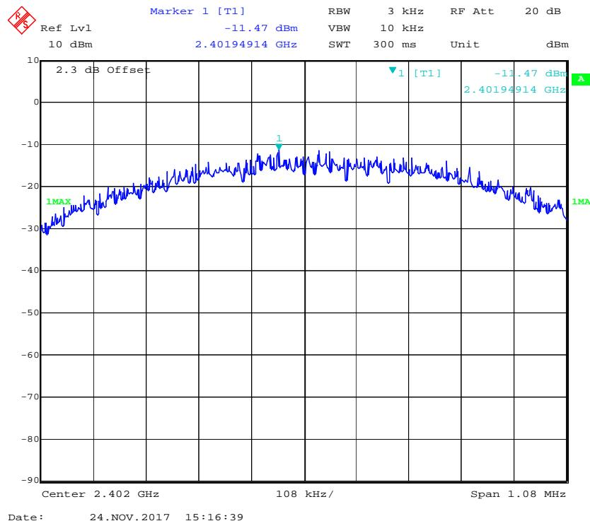
**Power Spectral Density, Middle Channel**
