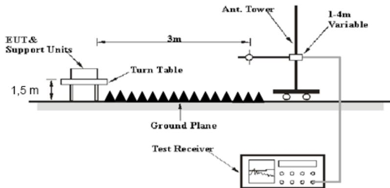
The radiated emission tests were performed in the 3 meters chamber test site, using the setup accordance with the ANSI C63.10-2013. The specification used was the FCC 15.209, and FCC 15.247 and RSS-247 §5.5,RSS-Gen §8.10 limits.
