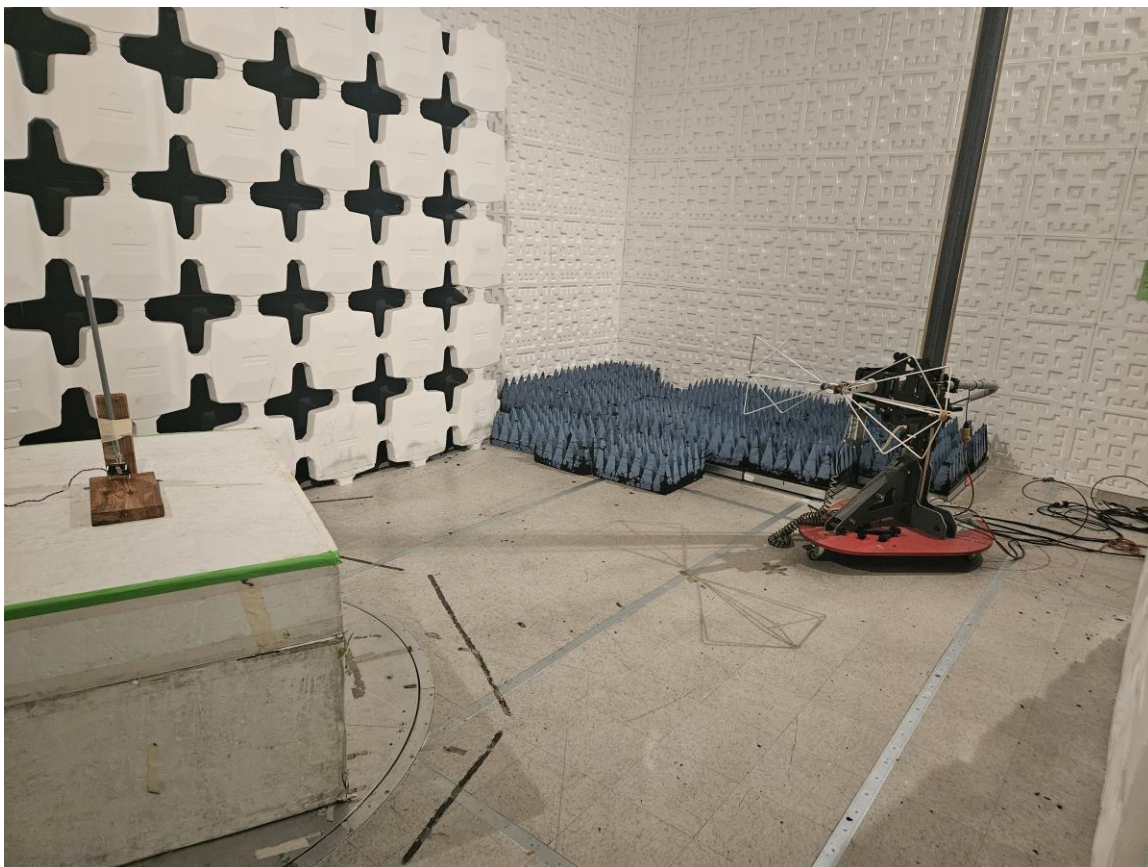
Figure 3. Radiated Emissions Test Setup, 30 MHz to 200 MHz
