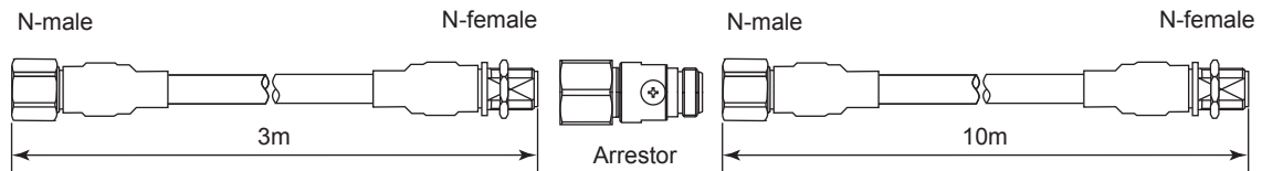
Figure 1-2 F9915KV remote antenna cable (13 m)
