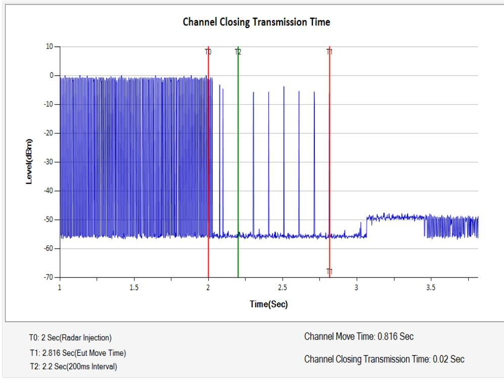
**Verdict:** Note: narrowing the sweep time as the good engineering process for the verification of transmission closing in 200ms
