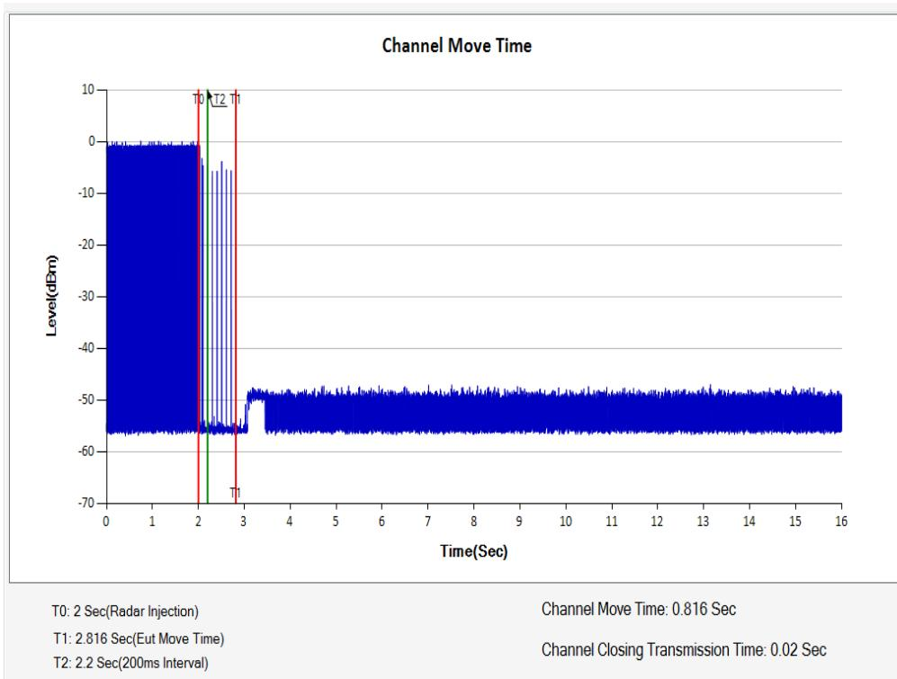
**Radar Type 1 Channel Closing Transmission Time**
