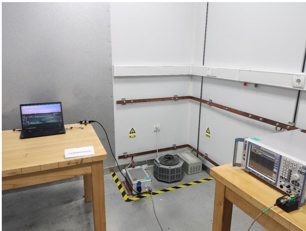
Conducted emission Test Setup
