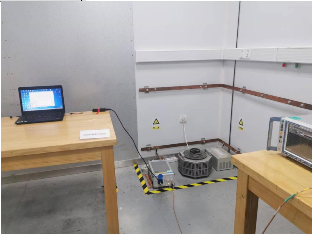
Conducted emission Test Setup
