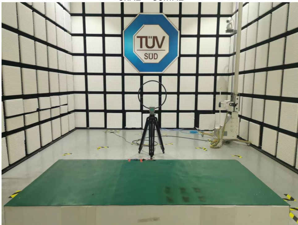
Radiated Emission Setup 9kHz ~ 30MHz
