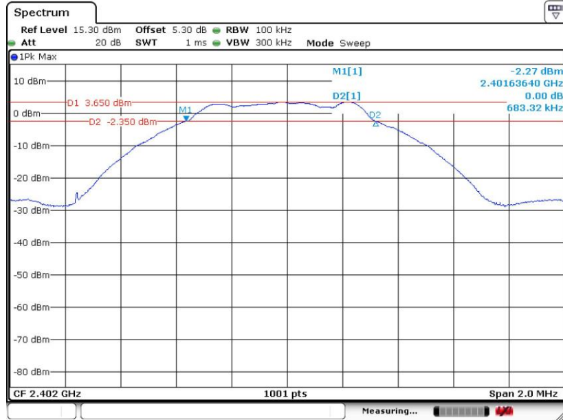
6 dB Bandwidth Plot on Channel 00
