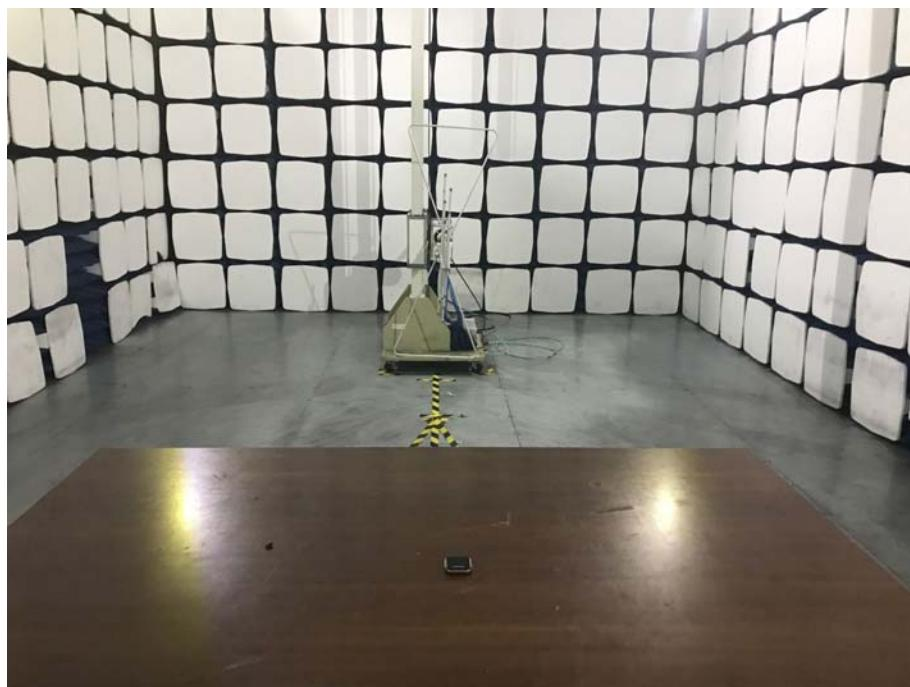
**Radiation Emission Test Setup (Above 1GHz)**
