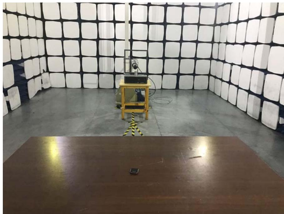
**Radiation Emission Test View (From 30MHz to 1GHz)**
