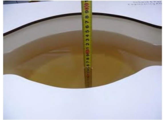
Liquid depth in the body phantom (835MHz)
