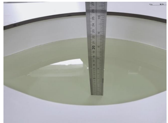
Liquid depth in the body phantom (2450MHz)
