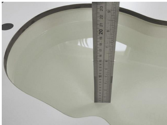
Liquid depth in the head phantom (2450MHz)
