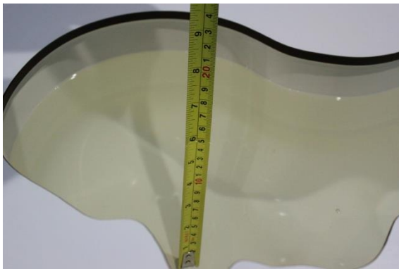
Liquid depth in the head phantom (1900MHz)
