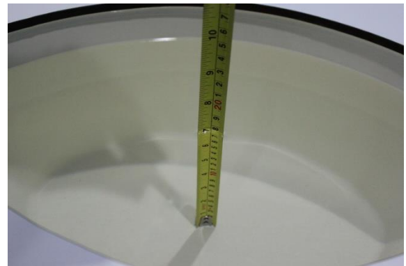
Liquid depth in the body phantom (1900MHz)
