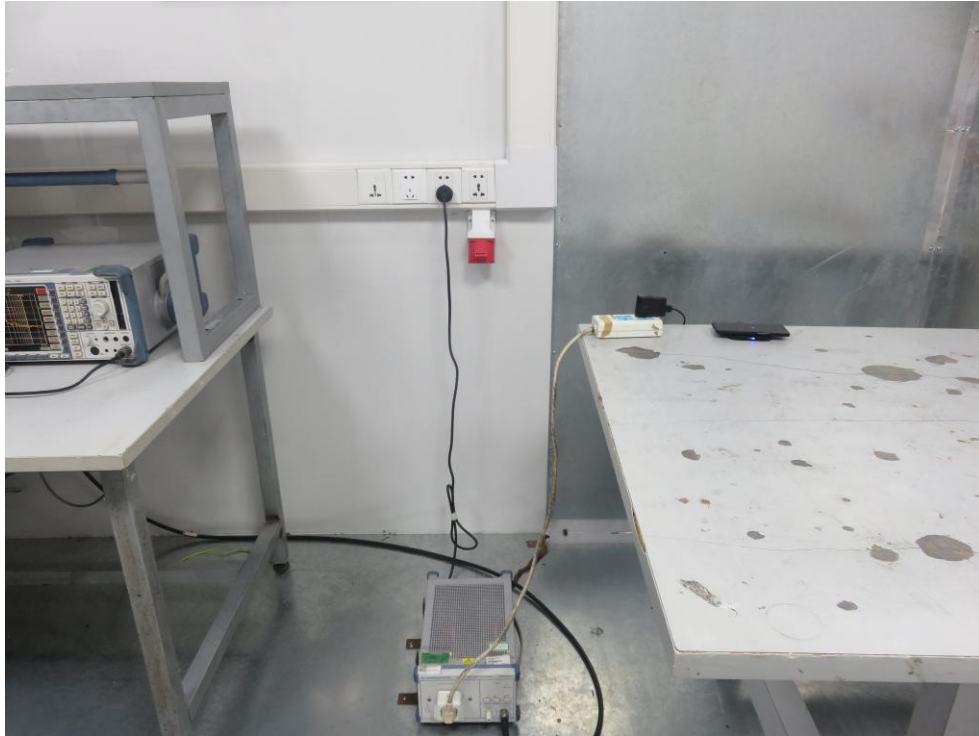
Photo of Conducted Emission Measurement
