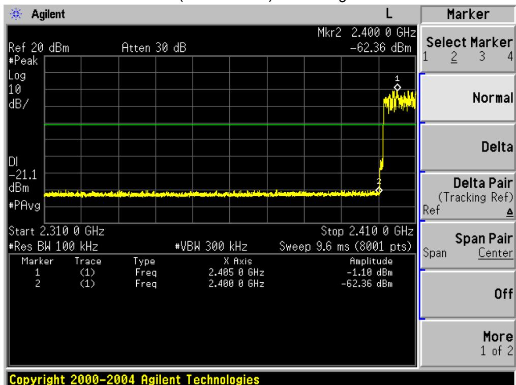
EDR mode ( $\pi/4$ -DQPSK): Band Edge-Right Side
