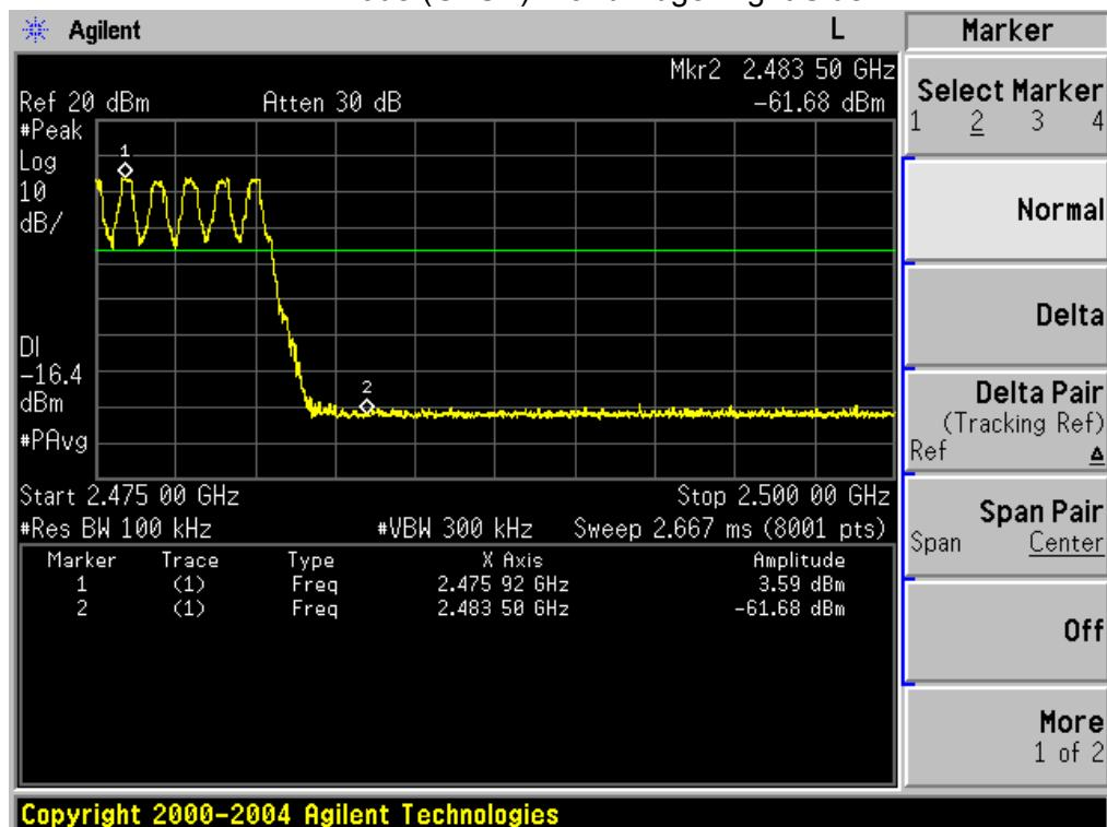
EDR mode ( $\pi/4$ -DQPSK): Band Edge-Left Side
