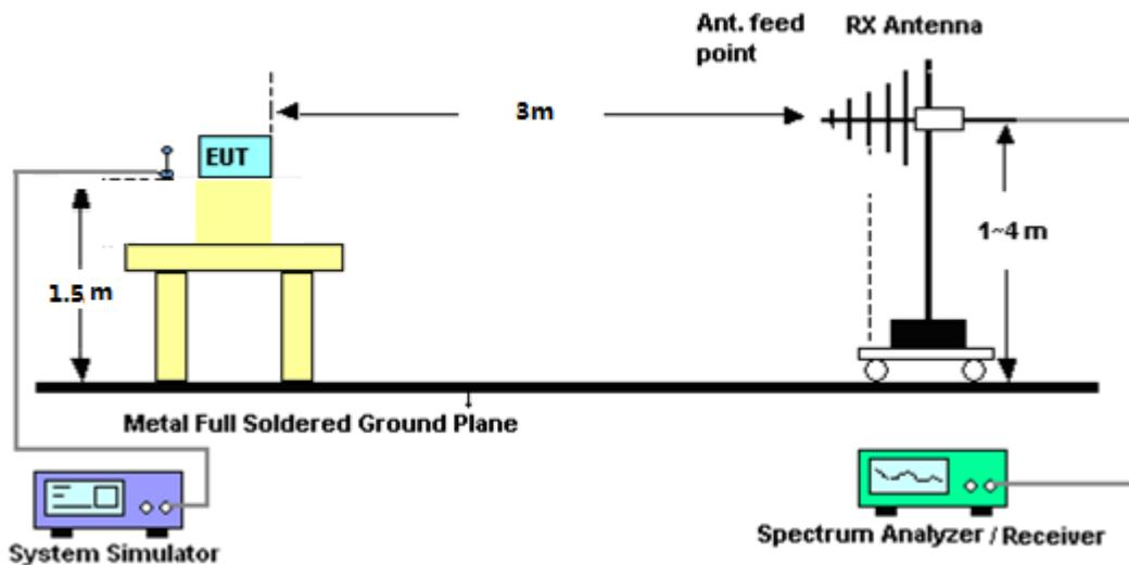
For radiated test from above 1GHz
