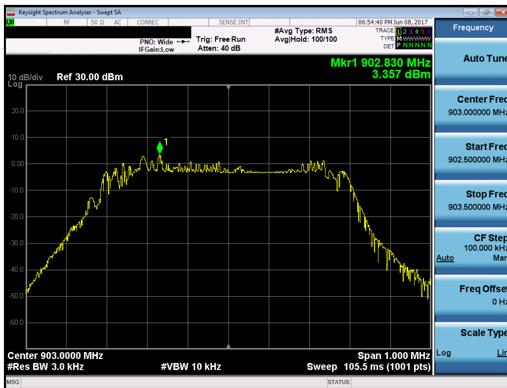
Plot 7-13. Power Spectral Density Plot (Low Channel)
