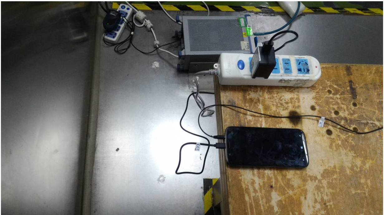
Conducted Emissions - Side View
