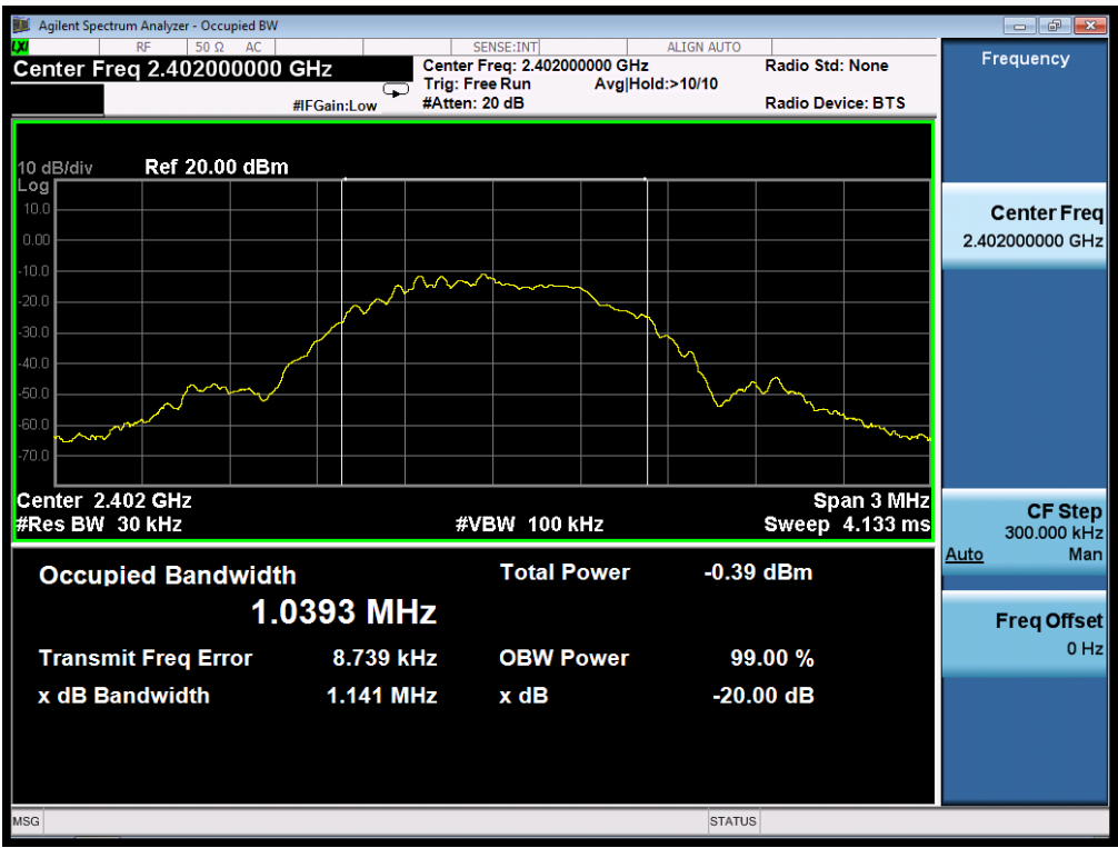
TEST PLOT OF BANDWIDTH FOR LOW CHANNEL
