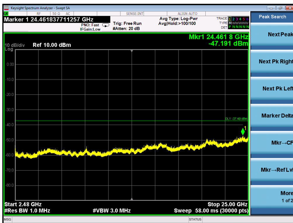
TEST PLOT OF OUT OF BAND EMISSIONS THE WORST CASE OF 802.11n20 FOR MODULATION IN MIDDLE CHANNEL
