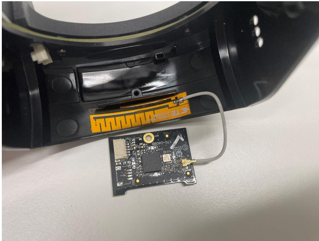
Internal Photo: Top of RF Board
