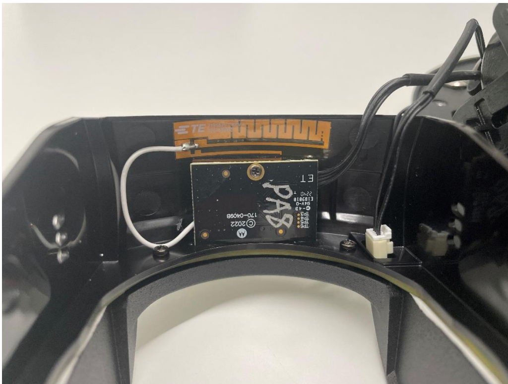
Internal Photo: RF Board & Antenna in Shroud
