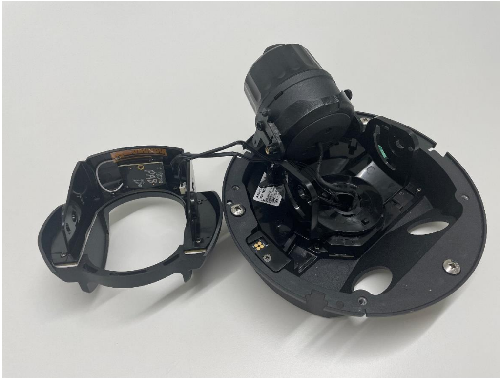
Internal Photo: RF Board & Antenna in Shroud
