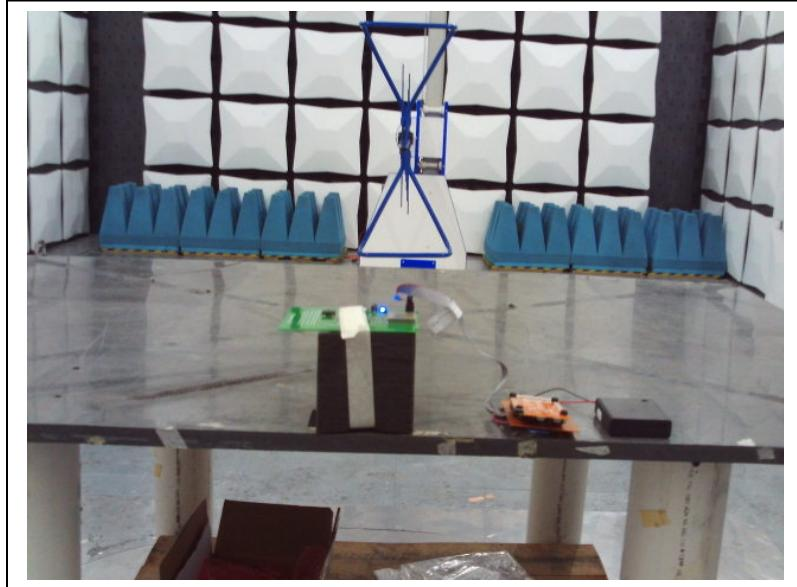
**Radiated Emissions: Loop Antenna, 0.009 MHz to 30 MHz**
