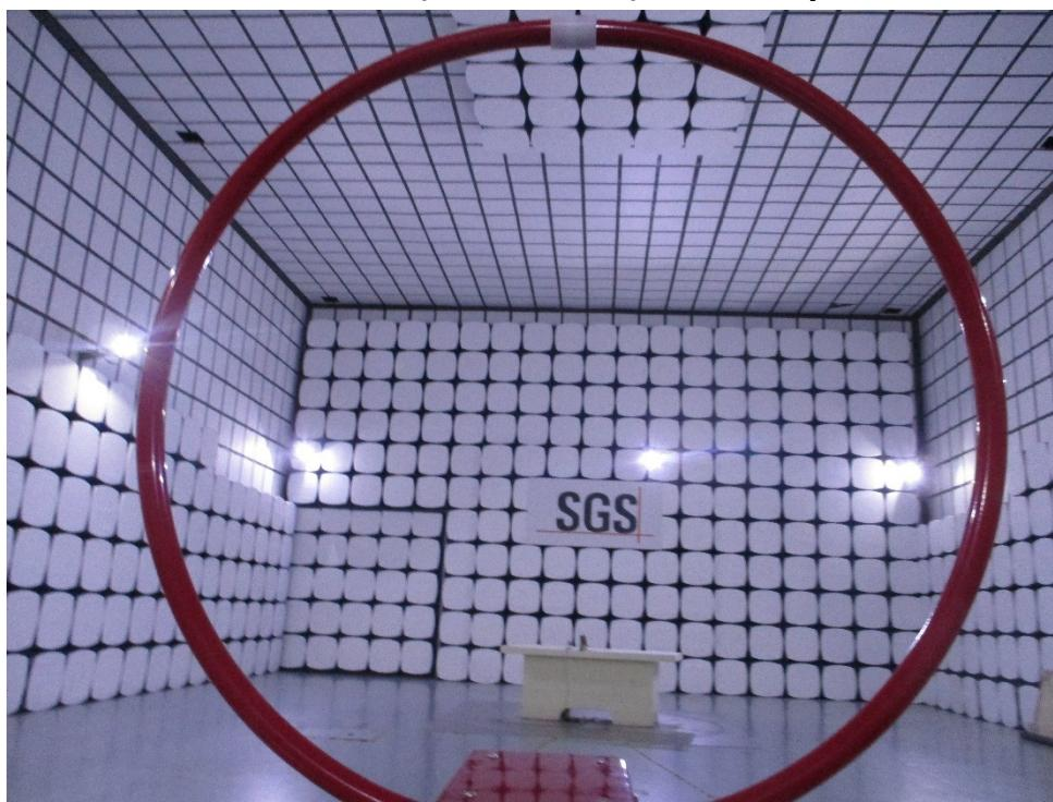
**8.3 Radiated Emissions(30MHz-1GHz) Test Setup**
