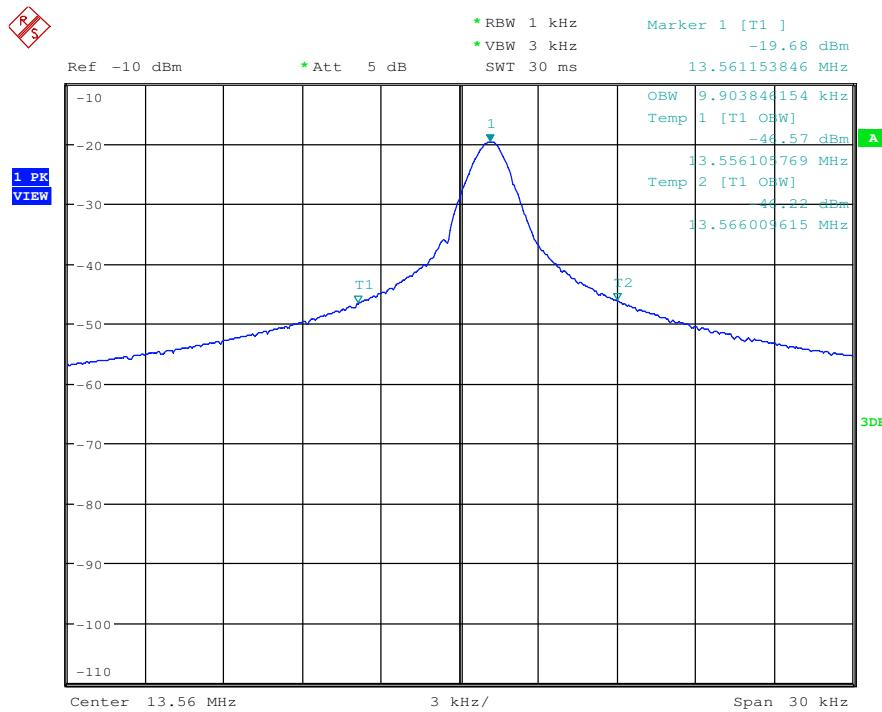
**7.5 Radiated Emissions(9kHz-30MHz)**
