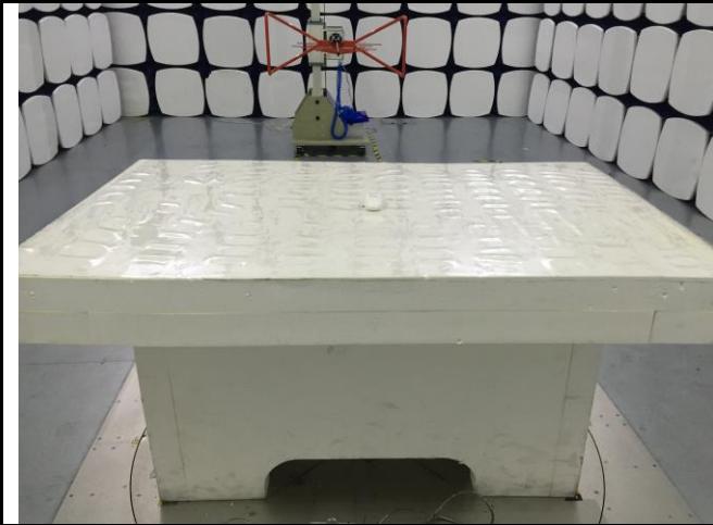
Radiated Spurious Emissions Test Setup Below 1GHz
