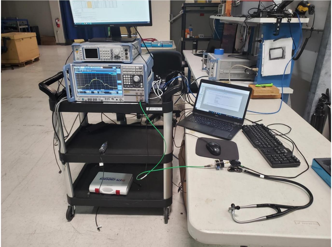
Figure 1 – Test setup (conducted)
