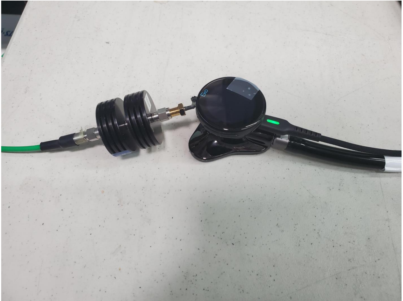
Figure 2 – Test setup, antenna conducted port, spurious emissions.
