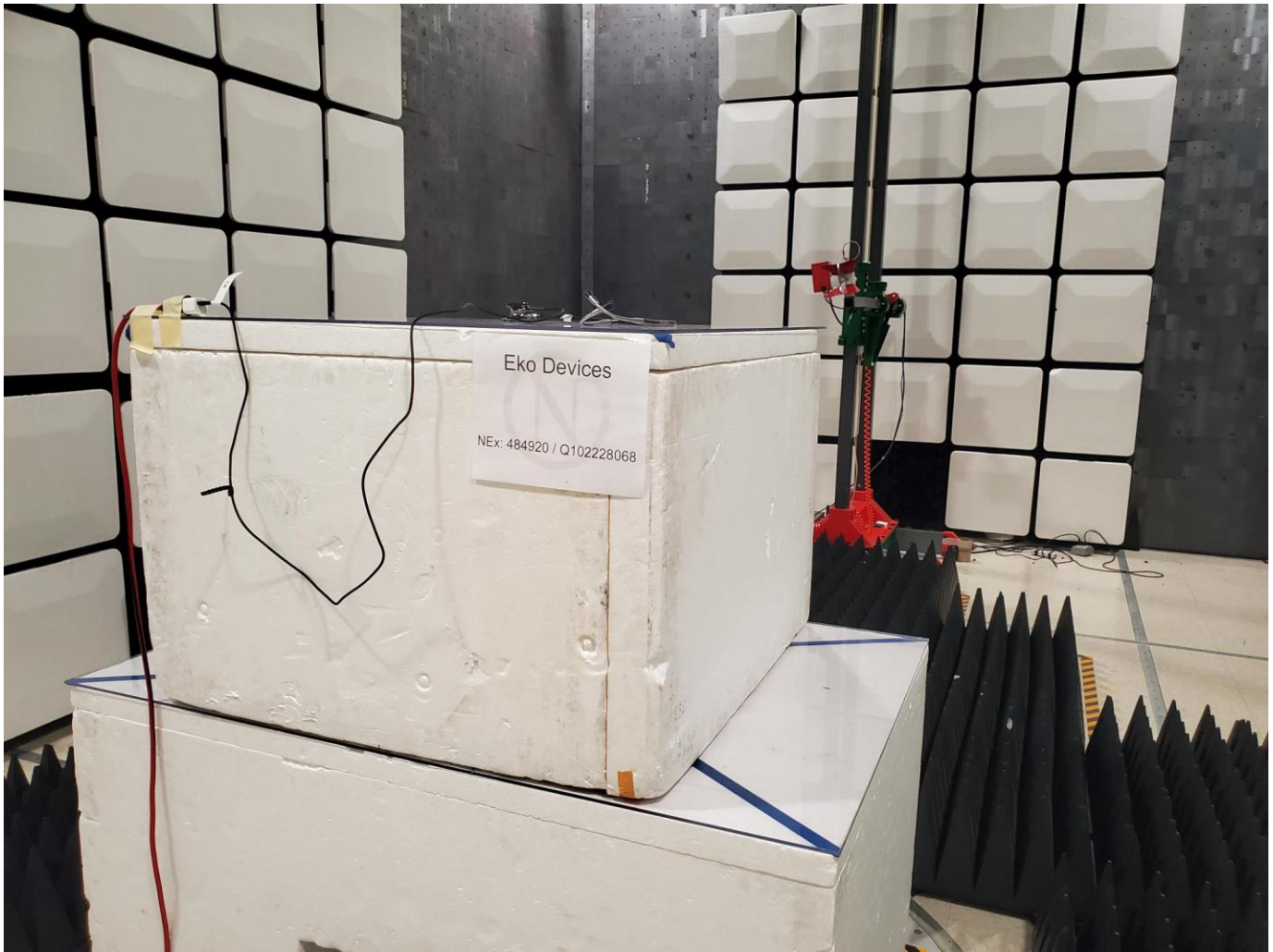
Figure 6 - Radiated emissions above 1 GHz (1 – 18 GHz), rear view.
