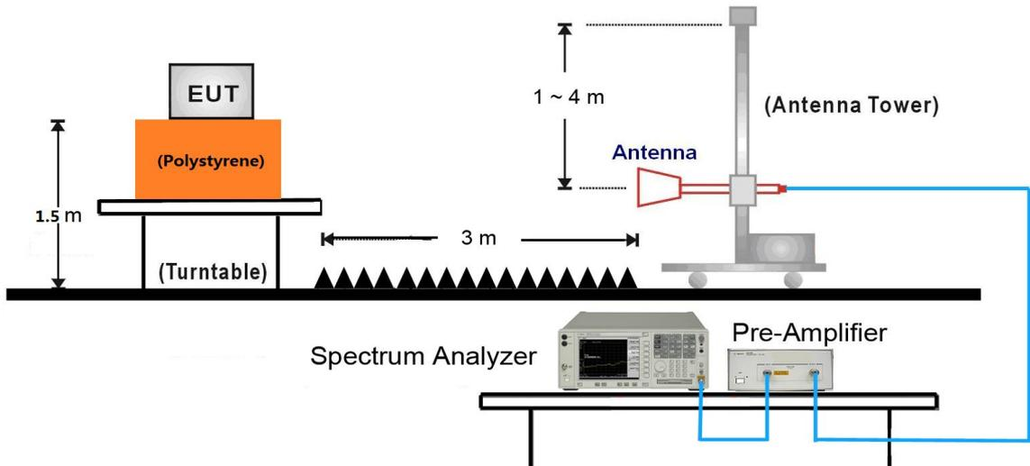
18GHz ~ 25GHz Test Setup:
