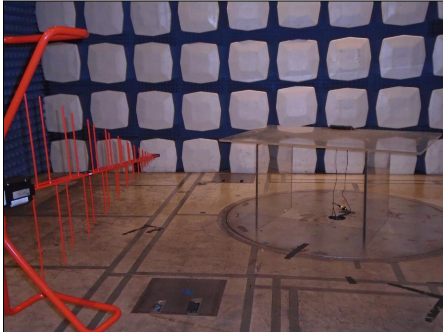
Photograph 1. Radiated Emissions, setup below 1 GHz
