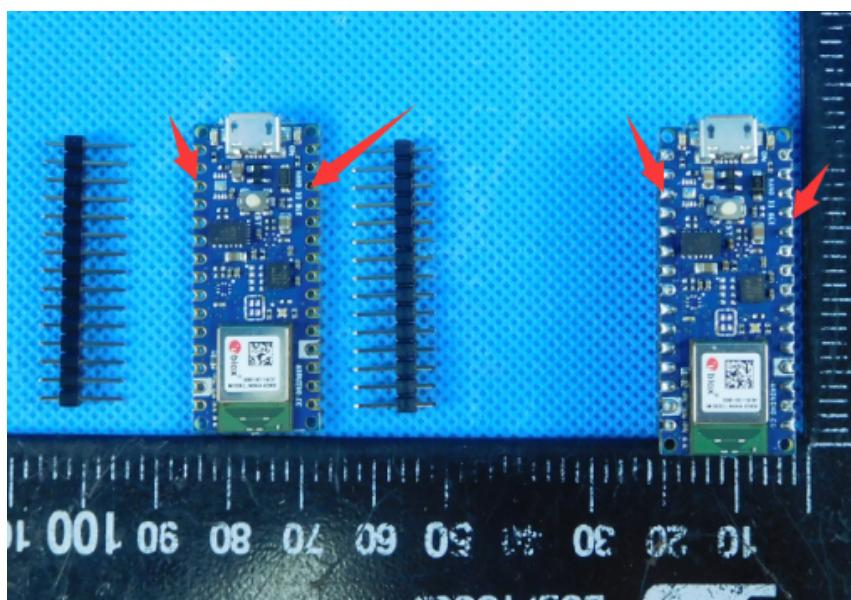
2.PCB layout between ABX00031/ ABX00035 and ABX00030/ ABX00034 models are different, one with sensor and one without. See the figure below for details
