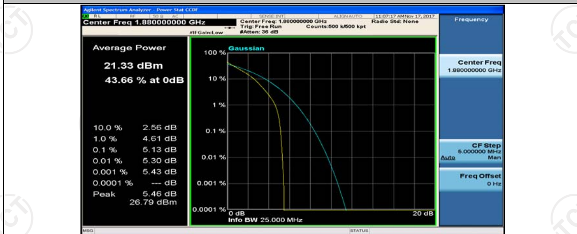
Channel Bandwidth: 10 MHz_MCH_QPSK_50RB#0
