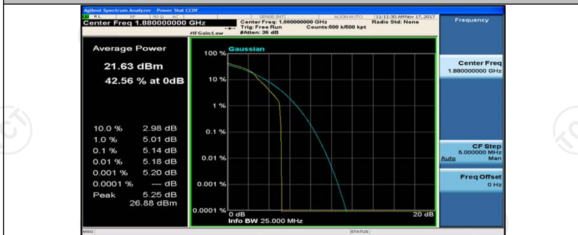
(Channel Bandwidth:15 MHz)_MCH_16QAM_1RB#37
