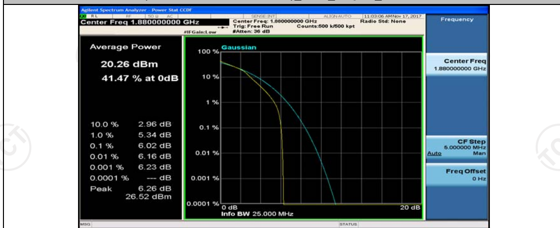
(Channel Bandwidth: 5 MHz)_MCH_16QAM_12RB#6
