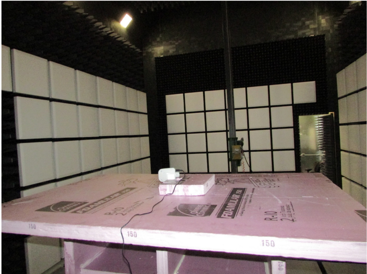
Figure 6: Radiated emissions >1GHz – Back view - Z-plane
