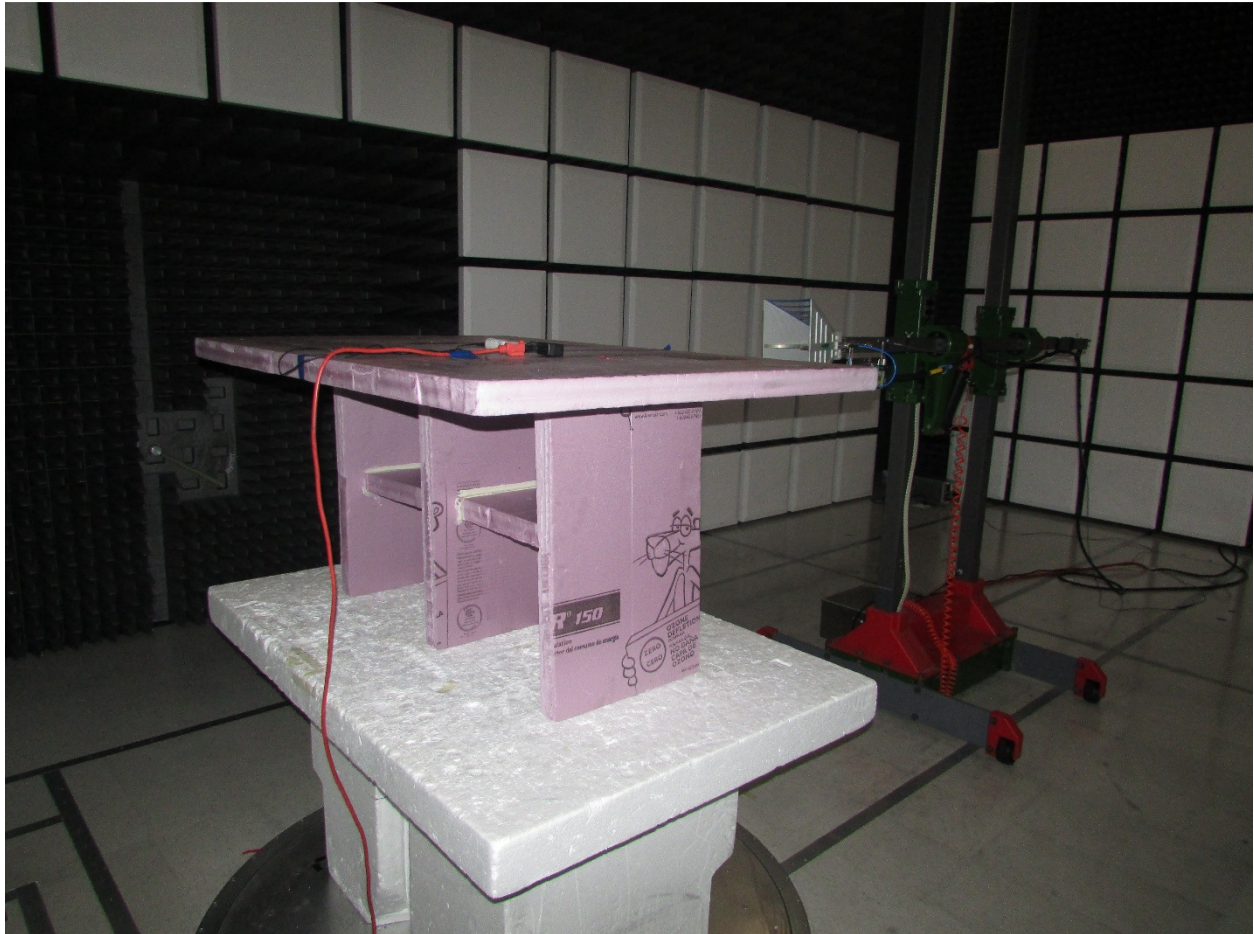
Figure 4: Radiated emissions >1GHz – Back view - X-plane
