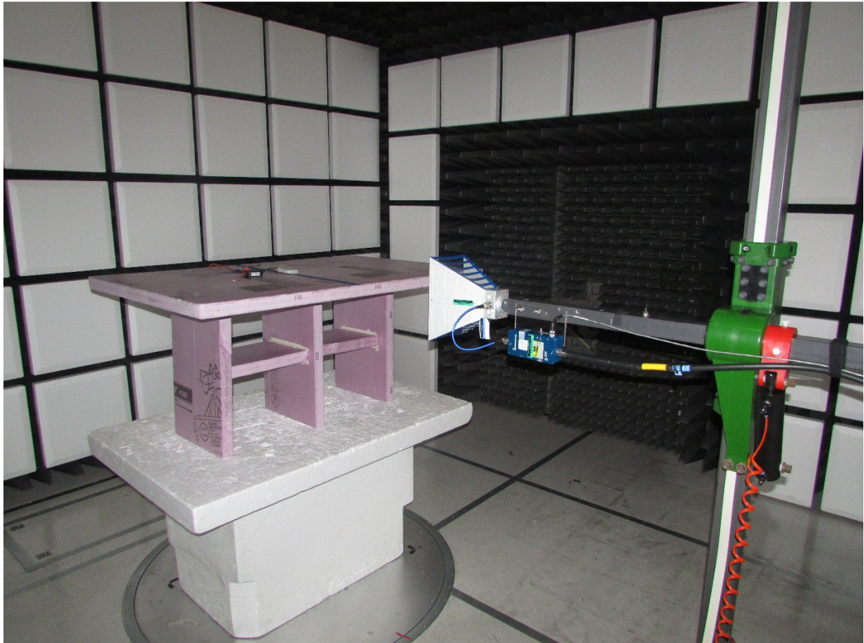
Figure 3: Radiated emissions >1GHz – Front view - X-plane
