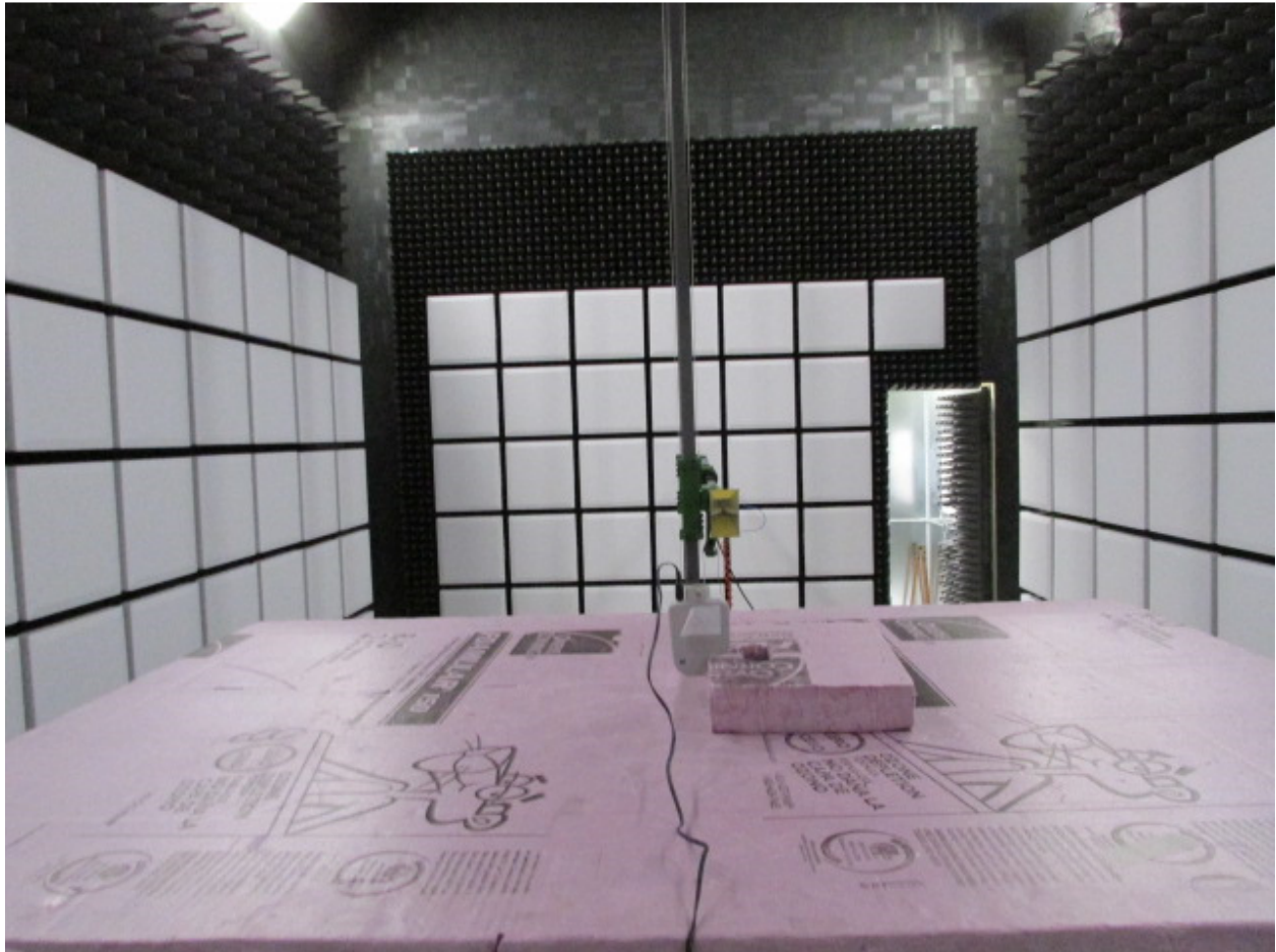
Figure 5: Radiated emissions >1GHz – Back view - Y-plane
