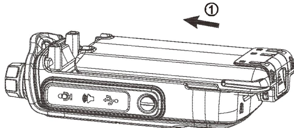
To remove the battery pack, pull upward the battery latch in the middle of the battery pack, then slide downward the battery away from the transceiver's body, and lift the battery from the transceiver's body.
