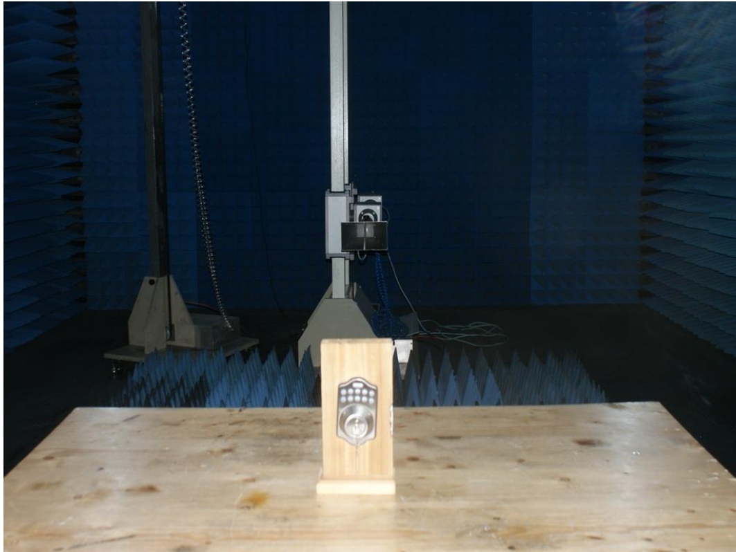
Photograph 7: Set-up for Radiated Emissions, above 1GHz
