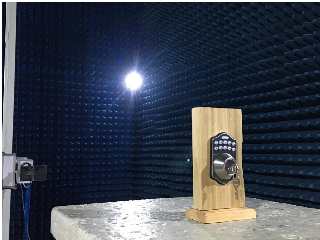
Photograph 4: Set-up for Spurious Emissions (1GHz-18GHz)
