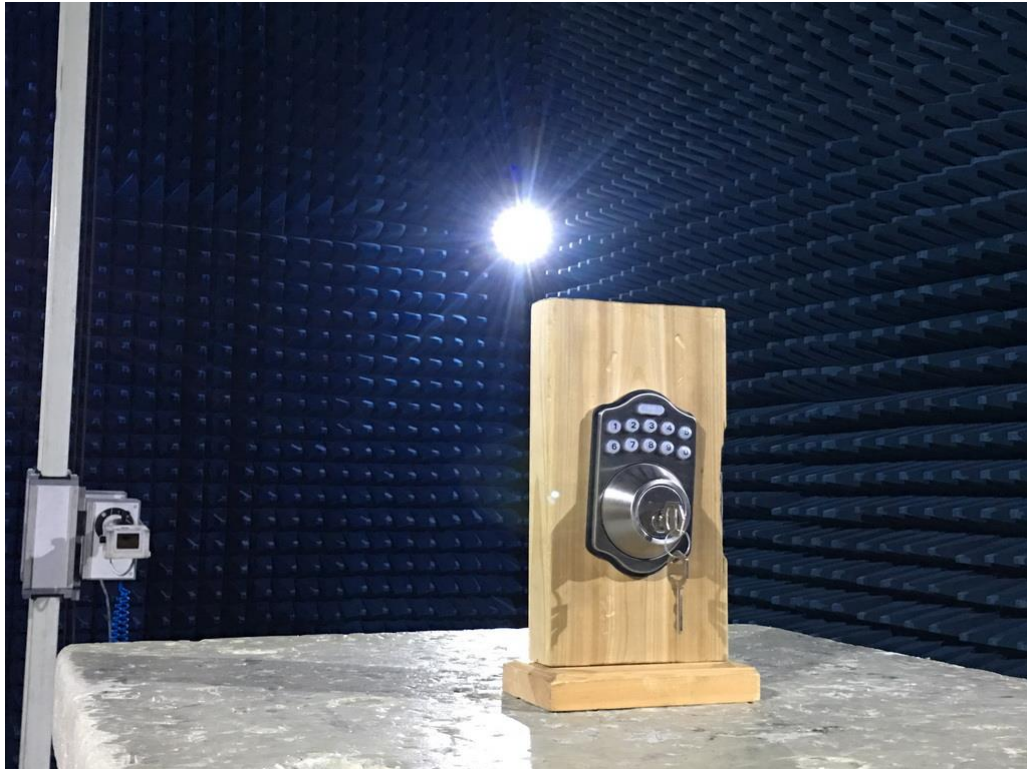
Photograph 5: Set-up for Spurious Emissions (18GHz-26GHz)
