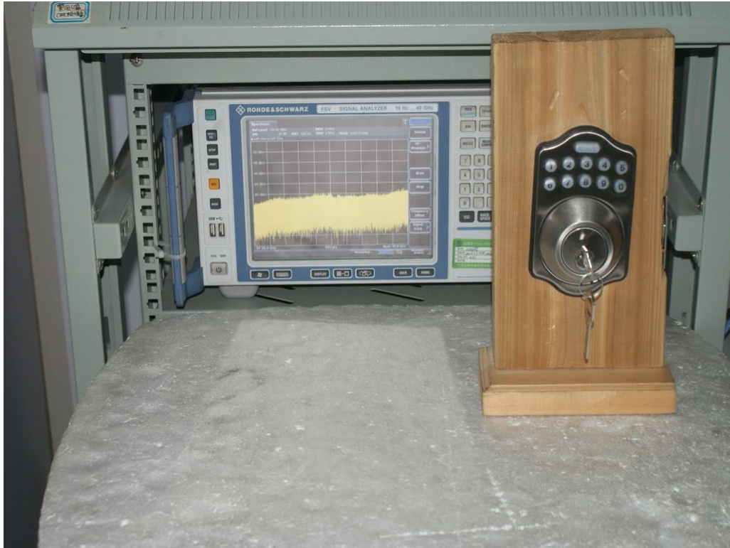
Photograph 1: Set-up for Radio Spectrum Test
