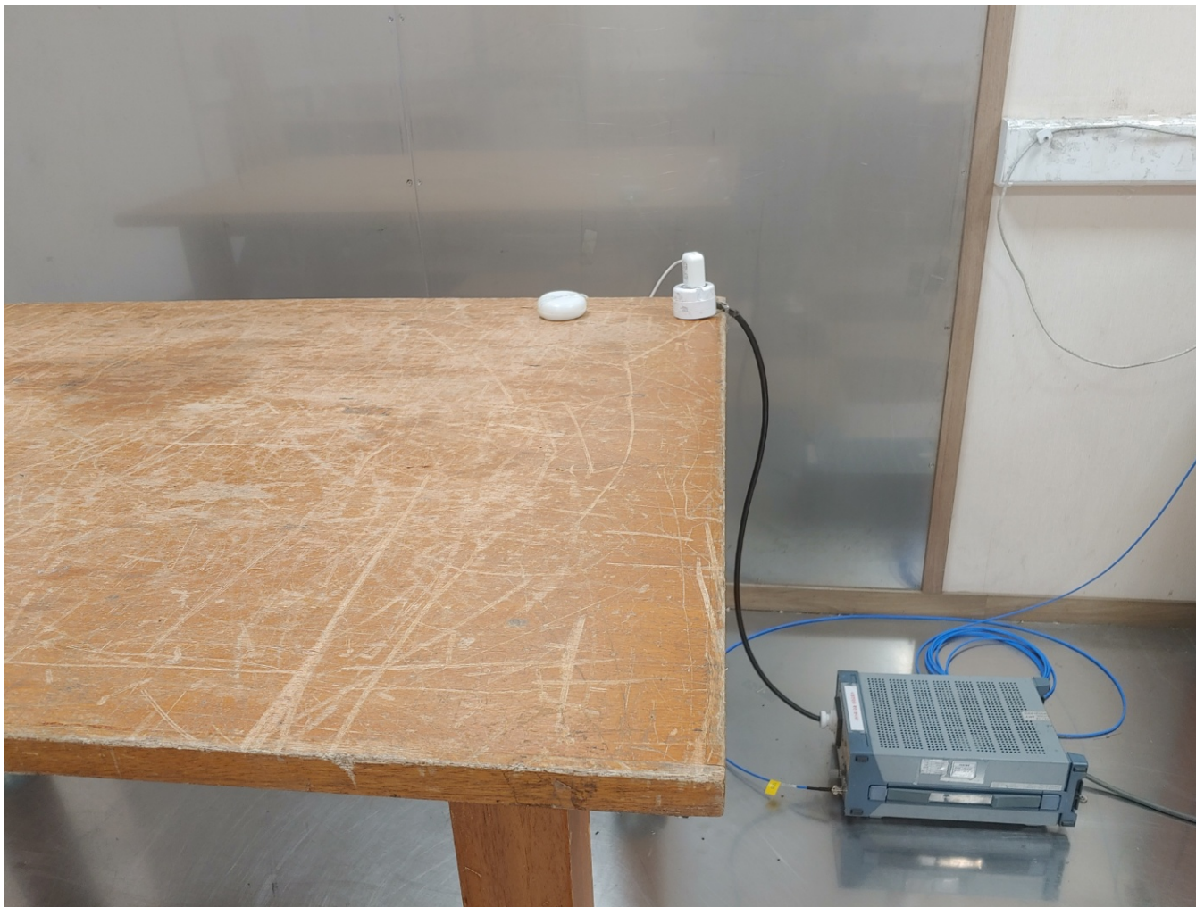
Conducted emission measurement (Front)
