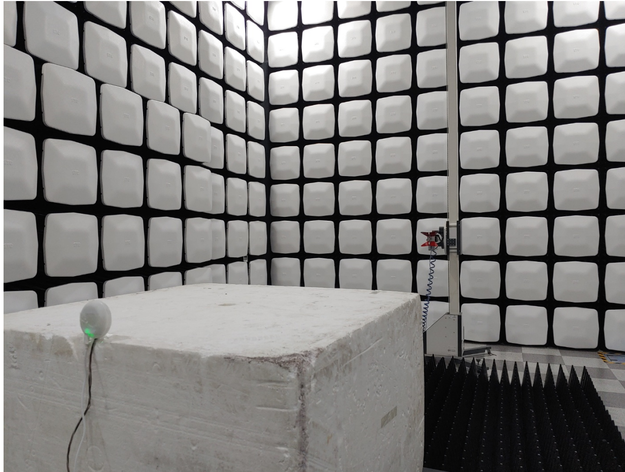
Radiated RF measurement (Above 1 GHz)_3m
