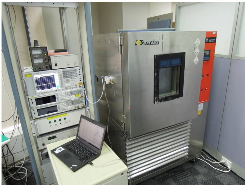
Photograph 5: Set-up for Conducted testing
