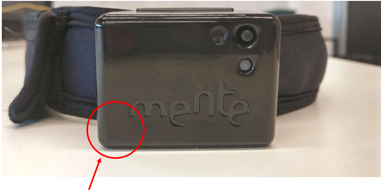
Photo 2: Antenna location (Front/Top view)
