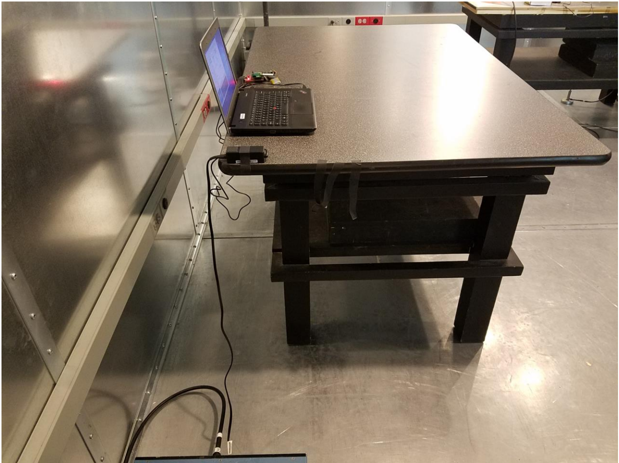
Figure 11: Conducted Emission Test Setup (Rear View)
