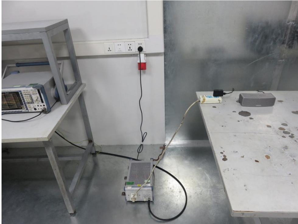
Photo of Conducted Emission Measurement
