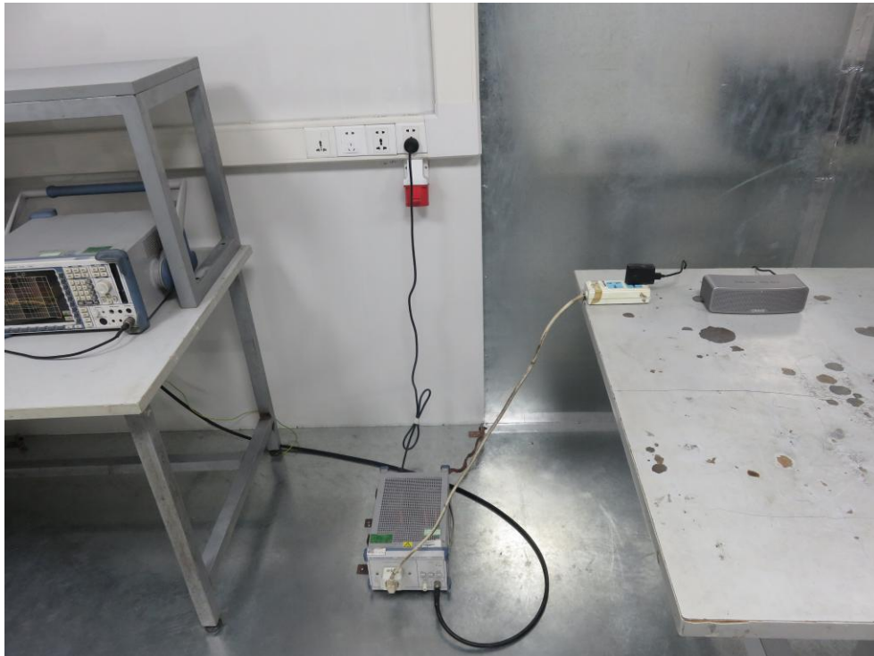
Photo of Conducted Emission Measurement
