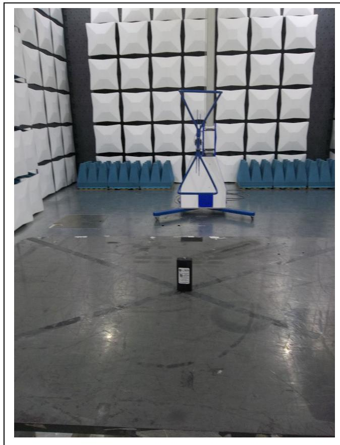
**Spurious Emissions, Battery Mode: 1 GHz to 18 GHz**
