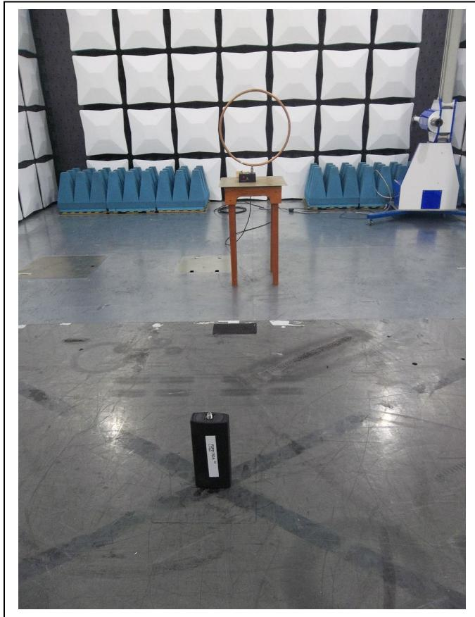
**Spurious Emissions, Battery Mode: 30 MHz to 1000 MHz**
