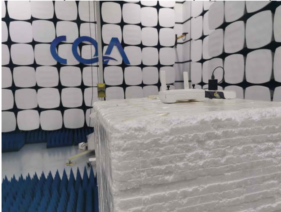
Radiated spurious emission Test Setup-3(Above 1GHz)
