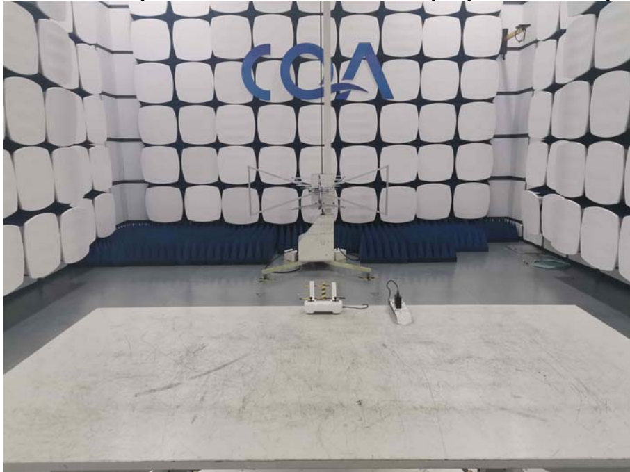
Radiated spurious emission Test Setup-2(30MHz-1GHz)
