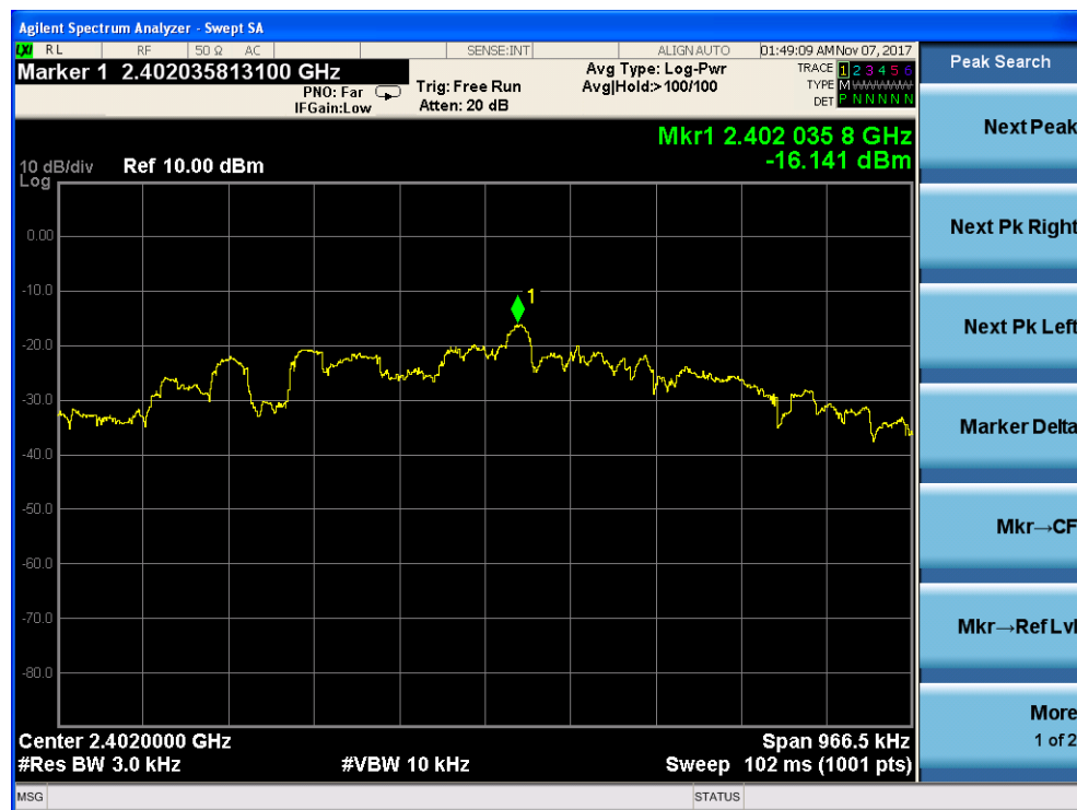
Power spectral density plot on channel 00
