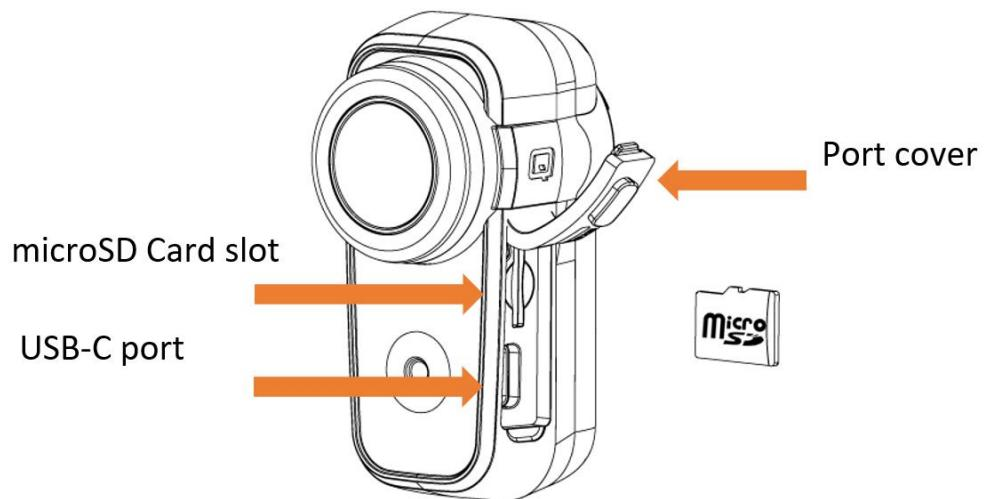
You can insert a microSD card into the microSD card slot of your Fly6 device and press in gently until locked in place. Please ensure the label on the microSD card is facing towards the front of the Fly6, as illustrated above.
