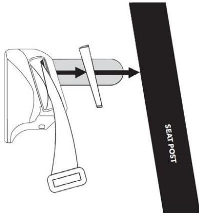
3. While holding the seat post mount against your seat post, wrap the seat post strap around the seat post and pull through the slot at the other end of the Fly6 seat post mount.
