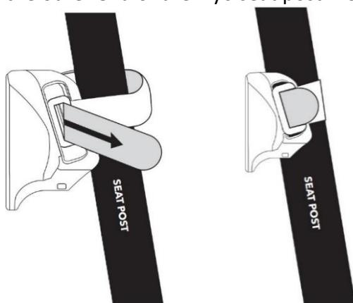
4. To mount your Fly6 align the tabs on the device with the slots in the seat post mount. Turn device **clockwise** a 1/8th turn until you hear a click and then the device will be locked into the seat post mount. Note : The device must be mounted in an upright position as shown.
