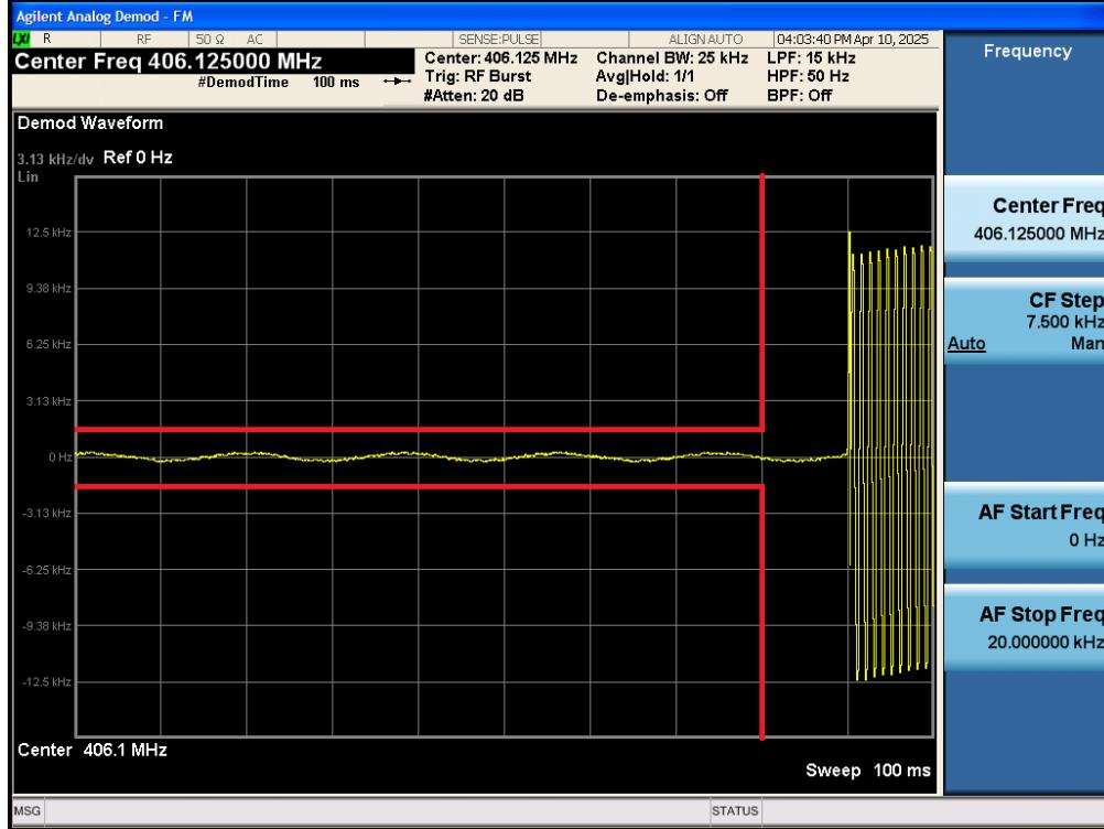
Note: All the test frequencies was tested, but only the worst data be recorded in this part.
