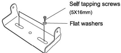
2. Fixed the radio and then insert the equipped with six angles combination screw and flat washers (each equipped with 2 sides and each side of 1 screw set) and tighten them.
