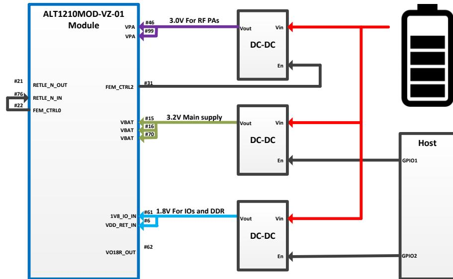
It requires additional supplies on application board, but allows shutting down the modem completely when not needed, therefore reducing the power consumption to minimum.
