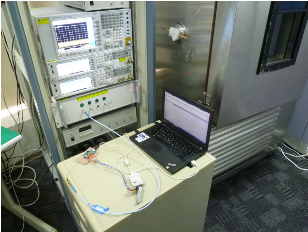
Photograph 5: Set-up for conducted measurement
